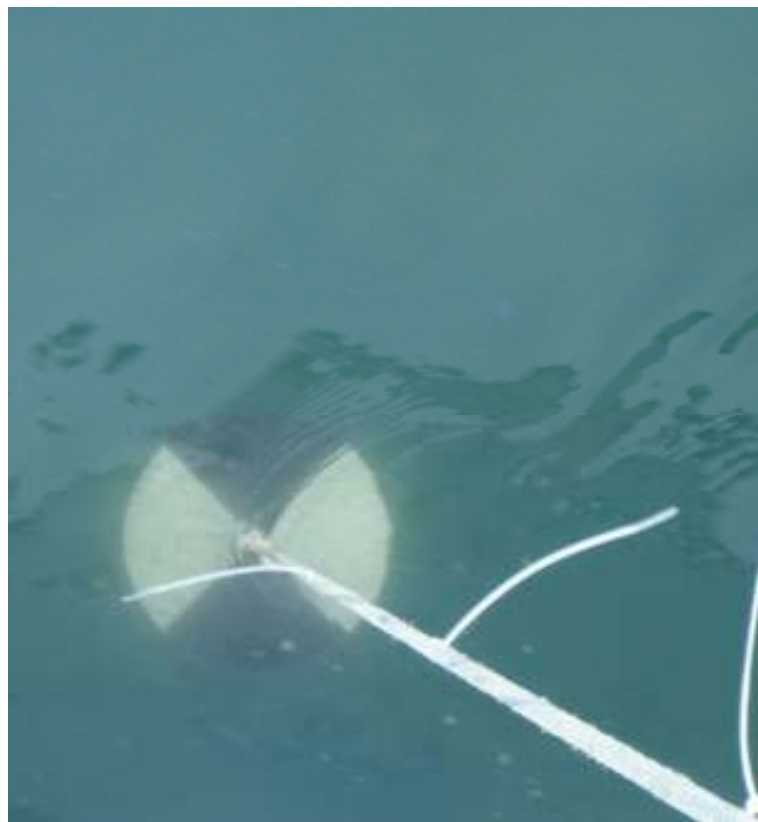
Figure 2. The employed Secchi Disk in the ROPME Winter cruise 2006.
